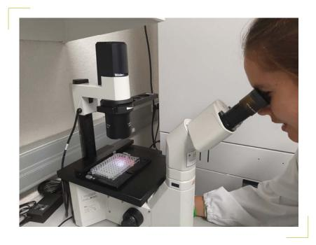
The Leica DMIL LED is versatile inverted microscope for cell inspection.
