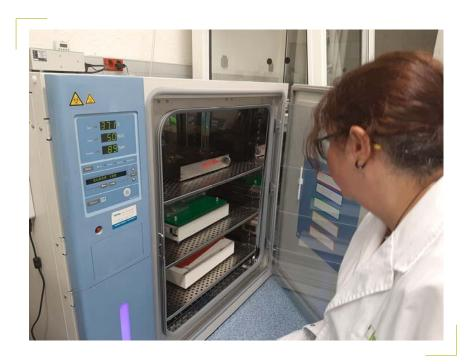
The Gadget Incubator is the largest capacity CO2 incubator available at the facility and features an active humidification system, HEPA filters and IR CO2 sensor for optimum cell viability.
